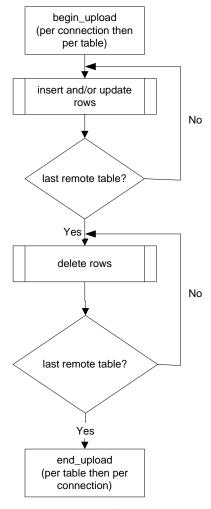
The end\_upload event marks the end of the upload transaction.
