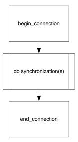
Following the synchronization, the connection is placed in a connection pool, and MobiLink again waits for a synchronization request for the current script version. Before a connection is eventually dropped from the connection pool, the end\_connection event is fired. But if another synchronization request for the same version is received, then MobiLink handles the next synchronization request on the same connection. There are a number of events that affect the current synchronization.
