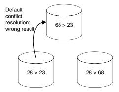
In this case the conflict should be resolved by summing the changes to the inventory column to produce the final result, so that a final value of 63 is placed into the database.
