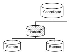
The following picture shows SQL Remote permissions, as granted at an internal site of a three-tier installation.
