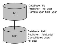
For any database in a SQL Remote replication setup, there are three permissions that may be granted to identify databases on the hierarchy:
