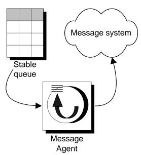
The transactions remain in the stable queue until confirmation has been received from all remote databases. When confirmation is received, the transactions are automatically removed from the stable queue by the Message Agent.
